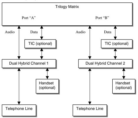
The Dual Hybrid module plugs into the second card slot of the frame, the first and third slots are for channel one and channel two Telephone Interface cards (TIC) respectively.
